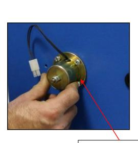
Electromagnet on the outer surface of the column
