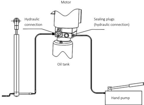
Figure: Hand pump connections
