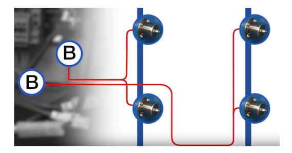
Figure: Electromagnet release connections
