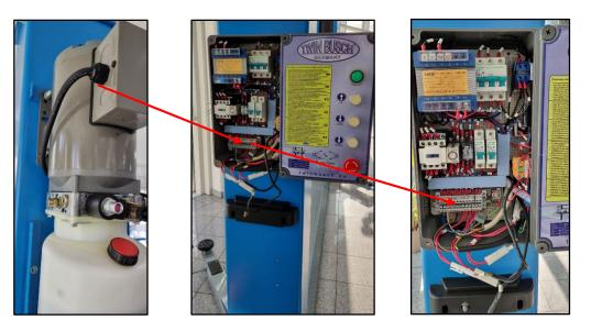
Figure: Connecting the power supply to the control unit
