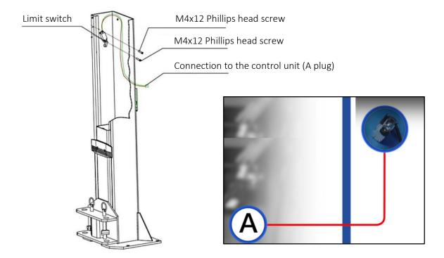
Figure: Mounting the limit switch
